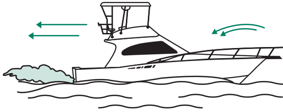
Figure 4. Engine or generator exhaust from your yacht while underway and operating with a high bow angle can cause excessive accumulation of Carbon Monoxide gas within the cabin and cockpit areas of your yacht. Always provide adequate ventilation and redistribute the load to lower the bow angle.
