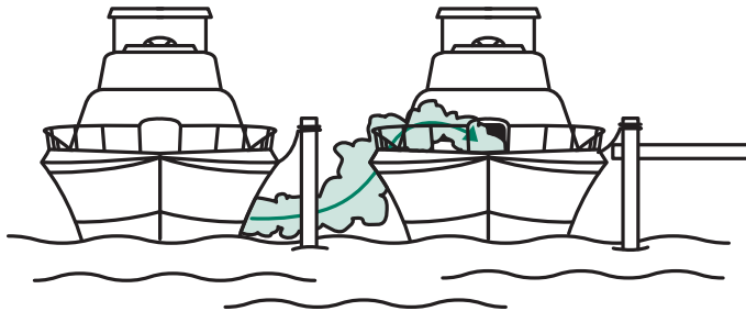
Figure 2. Engine and generator exhaust from other vessels alongside your yacht, while docked or anchored, can cause excessive accumulation of Carbon Monoxide gas within the cabin and cockpit areas of your yacht. Be alert for exhaust from other vessels.
