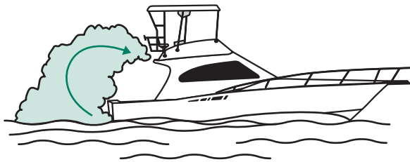
Figure 5. Engine or generator exhaust from your yacht while underway at a slow speed can cause excessive accumulation of Carbon Monoxide gas within the cabin and cockpit areas of your yacht. A tail wind can increase the accumulation. This is often referred to as the “station wagon effect”. Always provide adequate ventilation or increase your speed if possible.
